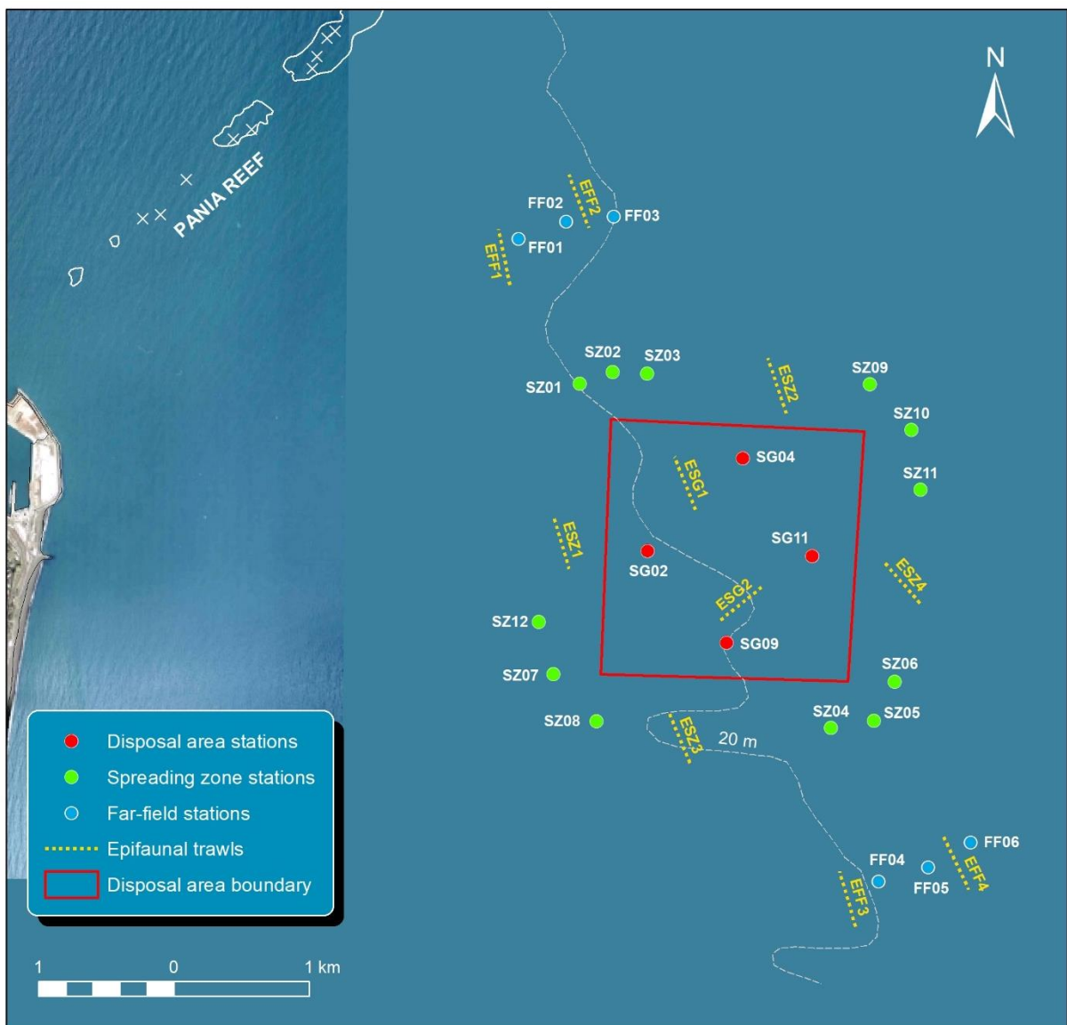
Figure 3. Spatial layout of principal sampling elements of the October 2021 survey; benthic grab stations and epifaunal dredge trawls. The 20-m depth contour from hydrographic chart NZ571 has been overlaid.
