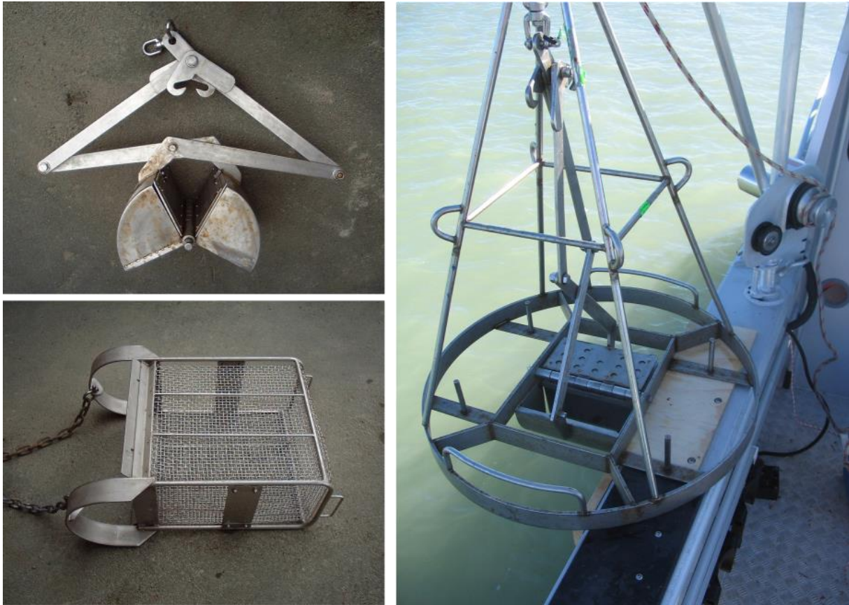
Figure 4. Top left: The van Veen grab sampler. Bottom left: The research dredge used to sample epifauna. Right: The grab sampler mounted in its frame.
